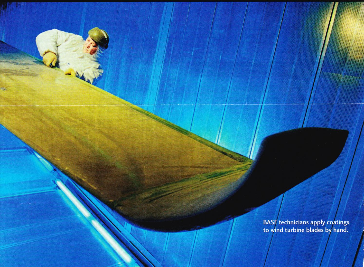
BASF technicians apply coatings to wind turbine blades by hand.
