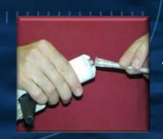
Attach large 6"nozzle by pressing in and twisting on.
