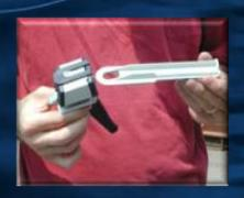
Remove nozzle from cartridge and wipe excess paint, reapply cartridge tip. Remove 2:1 plunger.
