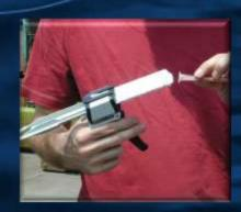
Attach small 3"nozzle by pressing in and twisting on.
