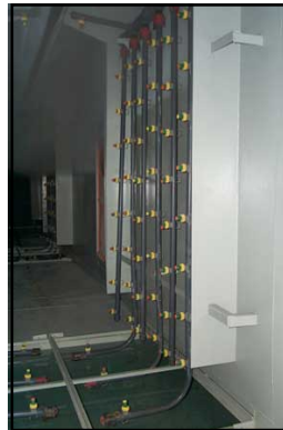
ACL’s stainless steel washer is resistant to the R.O water. The mild steel washer was internally sand blasted and coated with 20 mils of epoxy for protection.
