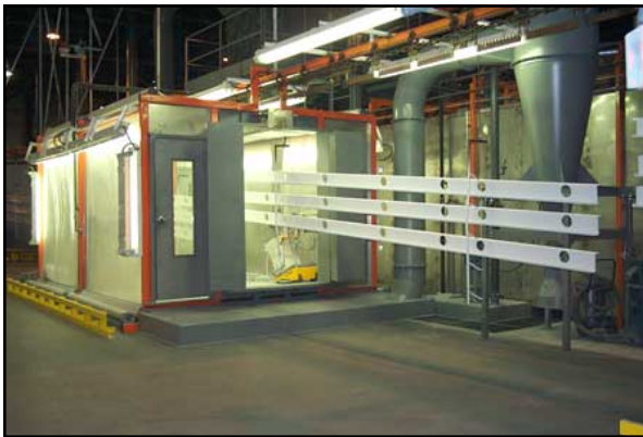
Coated extrusions are exiting the spray booth and will now enter the cure oven to complete processing.
