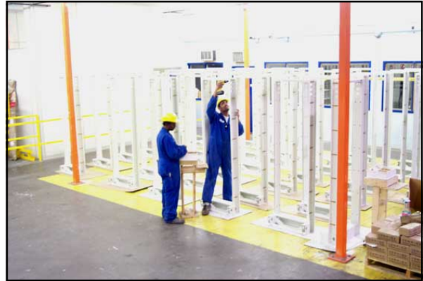
“Frame Assembly cell.” Bolt and torque various brackets and panels as per our customers drawings and requirements.
