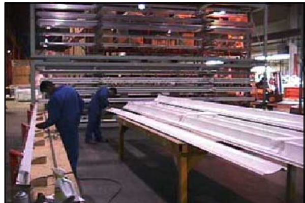
“Extrusion cell.” Clamp, punch and rivet these 22’ powder coated assemblies to customers drawings and specifications.
