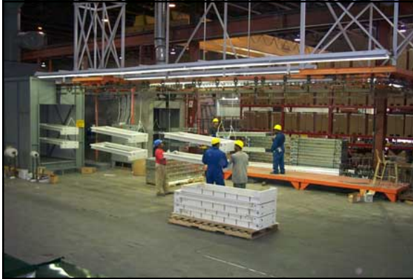
Line #2. Our large parts line (up to 35’ long) easily coats these 8’ frames to customers specifications.
